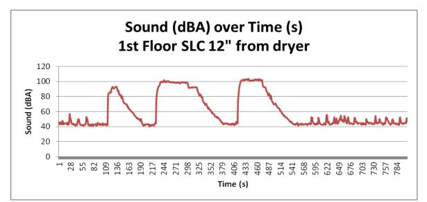
Figure 3: Hand dryer activated and left to run, activated and hands palms down, and then activated and hands cupped, palms up. (max 103.7 dBA)
