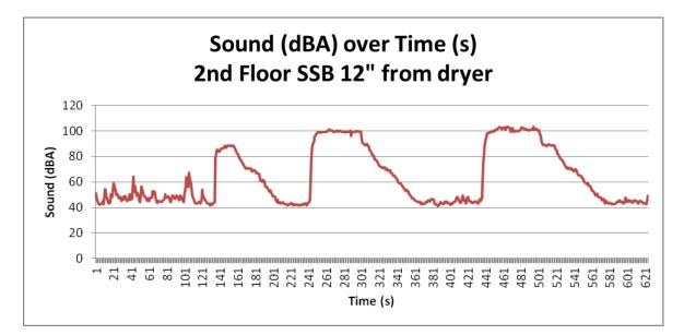
Figure 2: Hand dryer activated and left to run, activated and hands palms down, and then activated and hands cupped, palms up. (max 103.2 dBA)
