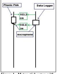
Figure 1 - Meter stick setup with sound monitor microphones aligned to the ear canal height of 143.6 cm.
